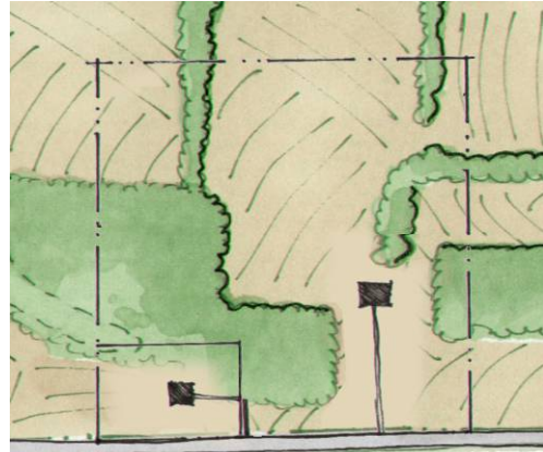
Step 1: A house with a private driveway and easement for extension of a private road
