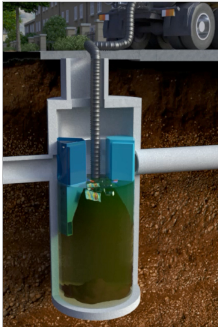
Fig.4 Floatables are removed with a vactor hose (First Defense model FD-4, shown).
