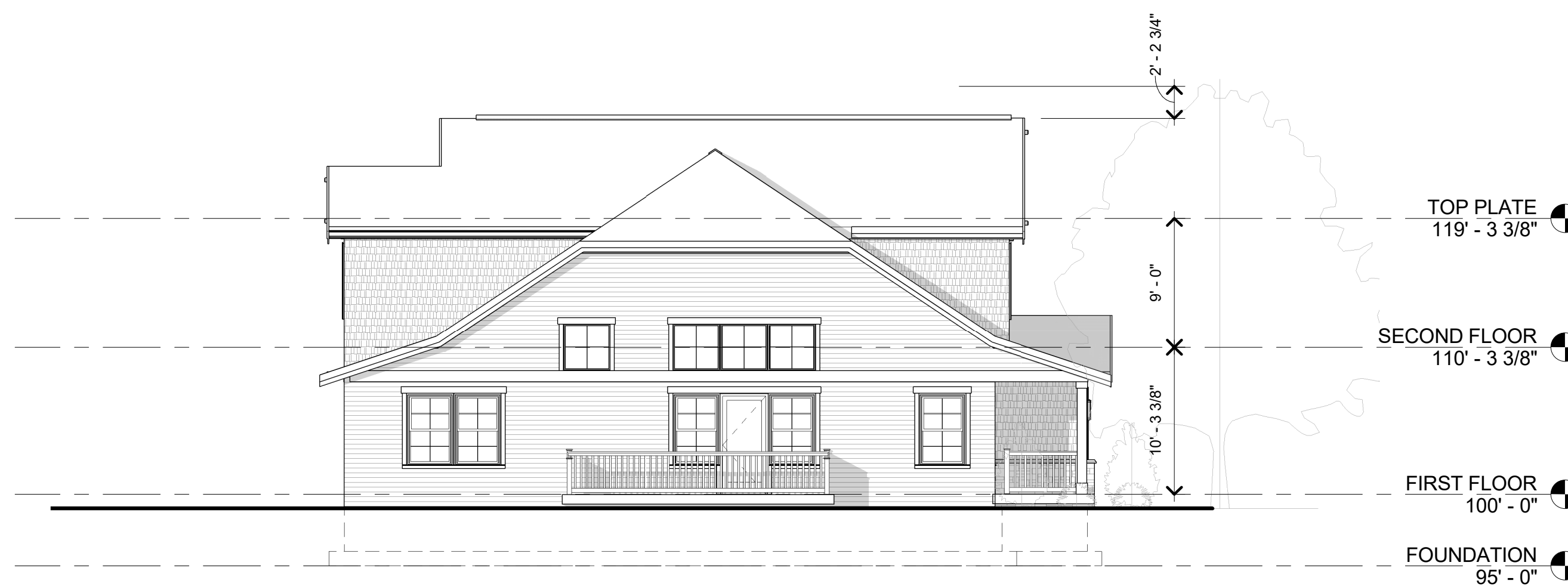
C6 ELEVATION - PROJECT WEST 1/8" = 1'-0"
