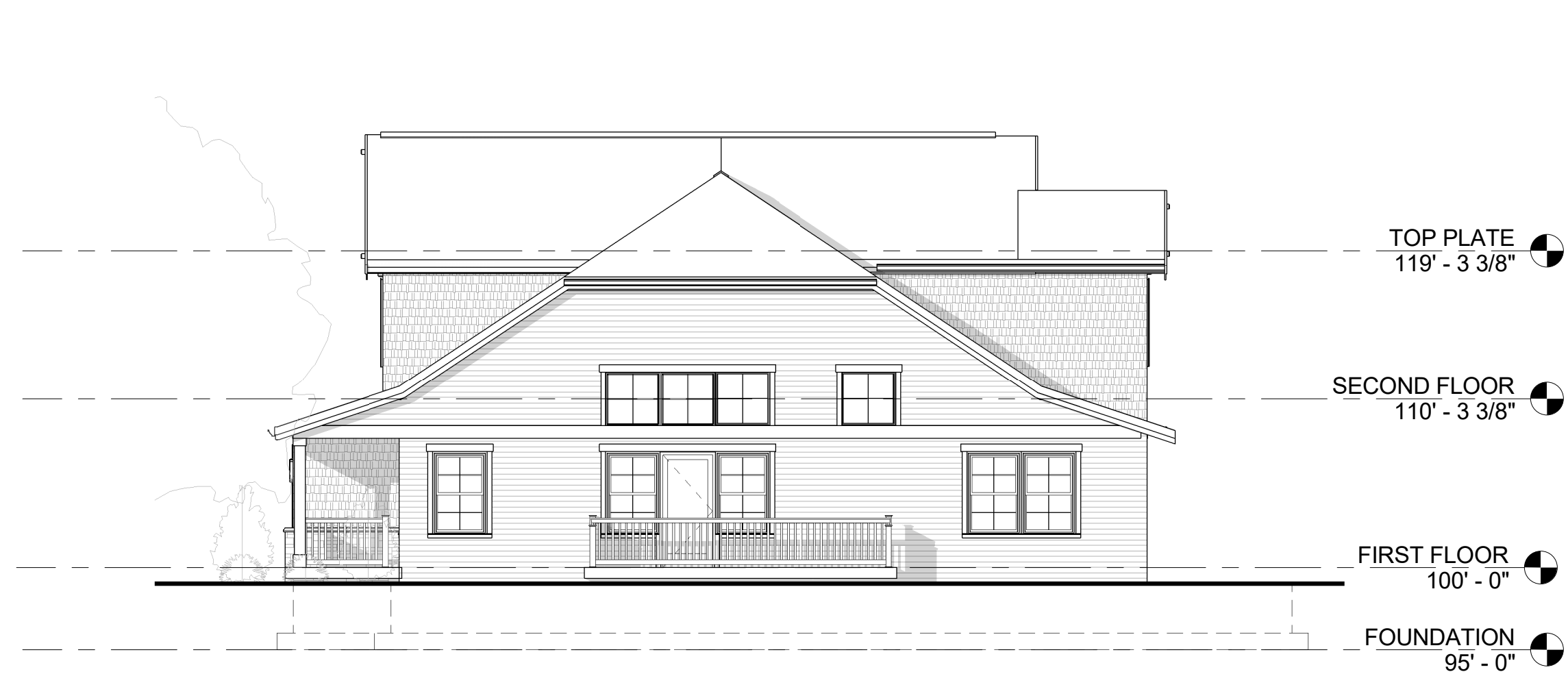
C2 ELEVATION - PROJECT EAST 1/8" = 1'-0"
