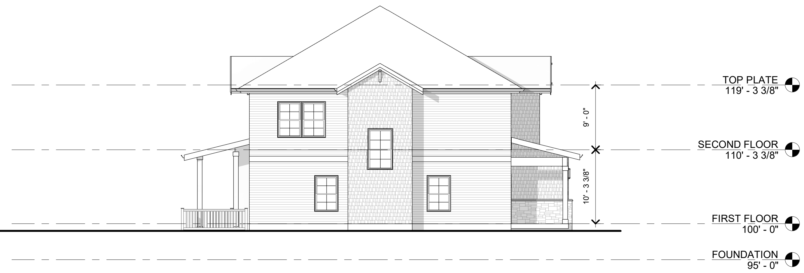
C6 ELEVATION - PROJECT WEST 1/8" = 1'-0"
