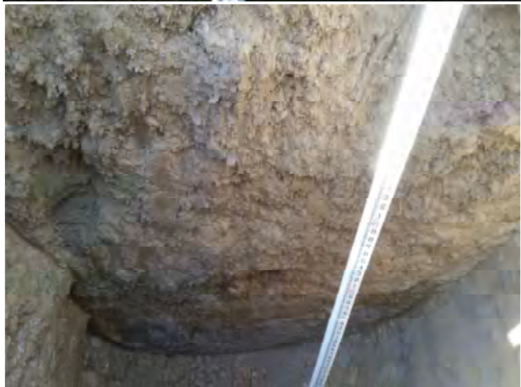
Photographs 25 and 26 (Top): Profiles of Test Pit TP-7. Photographs 27 (Bottom Left): Profile of Test Pit TP-7. At 10:30 AM water began to slowly seep in from sides and bottom of Test Pit. Photograph 28 (Bottom Right): Spoil Pile from Test Pit TP-7.
